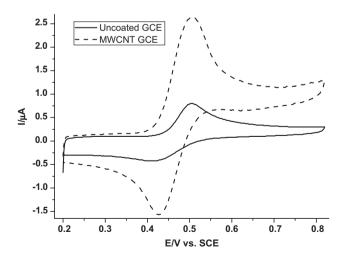
**Figure 1** Cyclic voltammograms of 98.0  $\mu$ M CAF on bare GCE (solid line) and MWCNTs/GCE modified electrode (dotted line) in 0.2 M phosphate buffer solution (pH 2.21) at a scan rate of 50 mV s<sup>-1</sup>.
