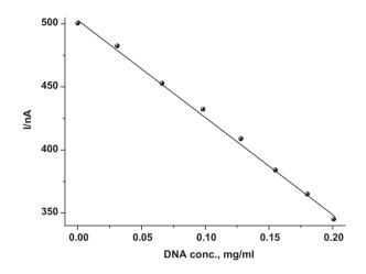
Figure 3 Dependence of the anodic peak current of CAF, 20.10  $\mu$ M, on the concentration of dsDNA at a scan rate of 20 mV s<sup>-1</sup>.
