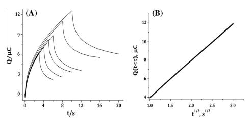
**Figure 4** Chronocoulograms of CAF, (A) and  $Q(t < \tau)$  versus  $t^{1/2}$  (B) in 0.2 M phosphate buffer solution (pH 2.21) at different duration times.
