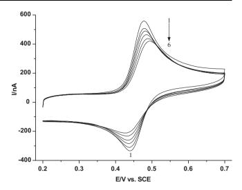
**Figure 2** Cyclic voltammograms of 20.1  $\mu$ M CAF at MWCNTs/ GCE in the absence and presence of DNA: (1) 0; (2) 0.0661; (3) 0.0982; (4) 0.128; (5) 0.155 and (6) 0.2 (mg ml<sup>-1</sup>) in 0.2 M phosphate buffer solution (pH 2.21) at a scan rate of 20 mV s<sup>-1</sup>.
