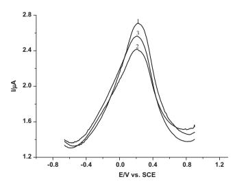
Figure 7 SWV of dsDNA-biosensor in 0.2 M phosphate buffer solution (pH 3.45), frequency = 50 Hz: (1) total oxidation of dsDNA-biosensor signal (maximum peak current), (2) immersion of the dsDNA-biosensor in a Fenton solution and (3) immersion of the dsDNA-biosensor in a Fenton solution with caffeic acid.
