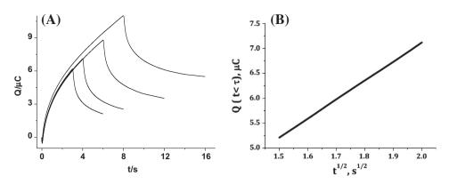
**Figure 5** Chronocoulograms of CAF-DNA, (A) and  $Q(t < \tau)$  versus  $t^{1/2}$  (B) in 0.2 M phosphate buffer solution (pH 2.21) at different duration times.
